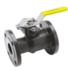
**88A-100 Series**—Carbon Steel Class 150 Flanged, regular port valves. Unibody to 2", easily-repaired split body 2-1/2" and larger. (88B series is unibody design 3" and 4"). Standard stem grounding and locking device. Includes ISO 5211 mounting pad. Meets all standards, including NACE when ordered with SS trim, and API 607 4th Ed, when ordered as –24. Available in 1-1/2"-10". (88B-100 Series 3" - 10" Regular Port, Unibody Design, ANSI Short Pattern)
